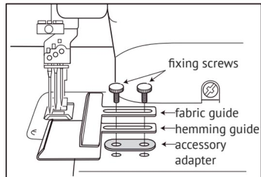
Accessory adapter and fixing screws are included with the machine
